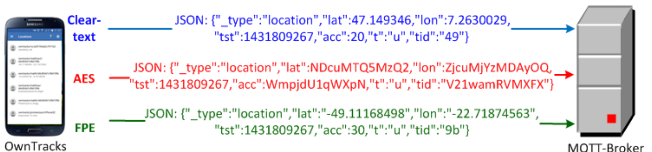
Figure 24: Content of the JSON in clear text, encrypted with AES or FPE
