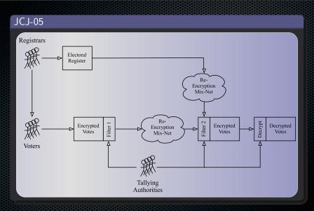
The modified scheme with time guarantee due to board flooding prevention
