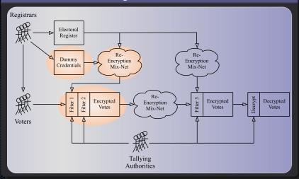
The modified scheme with time guarantee due to board flooding prevention
